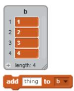
To add one more element to the list "b". The list element can be either numerical or text.
